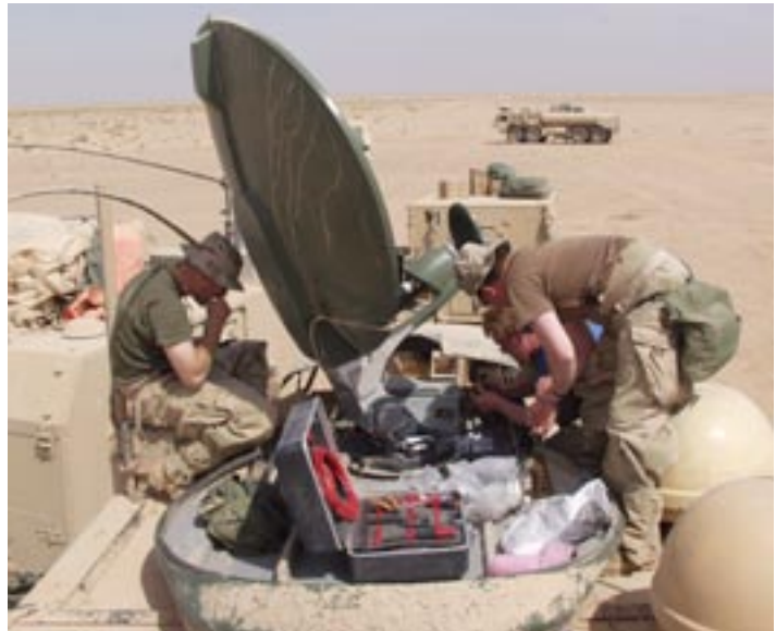
Central Iraq, SWE-DISH service technicians do a "500 km" check-up and change a wave guide on a DA150K Mil Drive-Away. The Drive-Away was used for command and control by the US Army Assault Command post during Operation Iraqi Freedom
